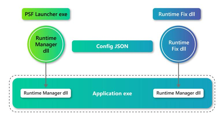
The above diagram explains the architecture of the Package Support Framework.
